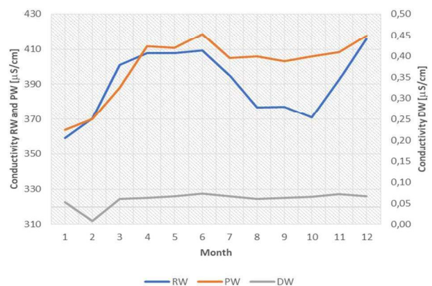
Fig. 2. Conductivity change at the different stages of production (RW-raw water; PW-pretreated water; DW-demineralised water).
